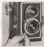
Setting the lever for flash synchronization with delay to peak (use only at 1/500 or 1/300)
