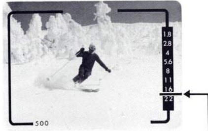
When camera is set at automatic, electric eye bar selects lens opening when shutter release button is pressed.
