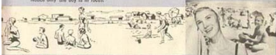
With a small lens opening, the sharpness range extends from near the camera to infinity, and everything is in focus.
