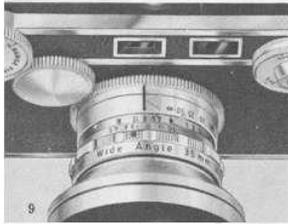
If the lens markings are not readily visible from the top of the camera—a convenience, not a necessity—the following adjustment may be made with a small jeweler's screwdriver. If you do not desire to make this adjustment, your local ARGUS Dealer can do it for you.
